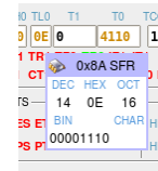
Figure 3.7: Representation of a register value in various numeric bases
