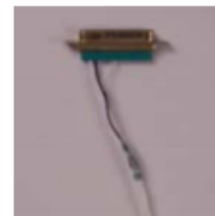
Coax Shield Terminated with Excessive Lead Length
