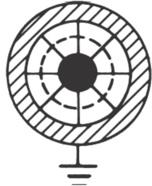
Fields around shielded conductor; shield grounded and carrying a current equal to the conductor current but in the opposite direction.
