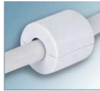
FIGURE 6-17. Magnetic material used as a shield by providing a low-reluctance path for the magnetic field, diverting it around the shielded region.
