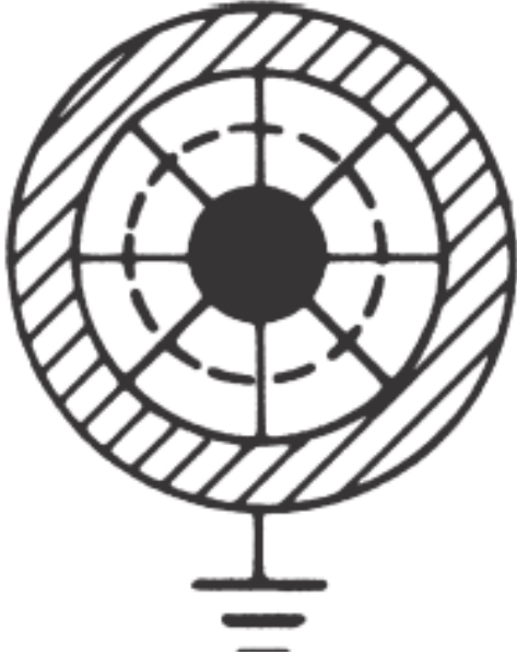
Fields around shielded conductor; shield grounded and carrying a current equal to the conductor current but in the opposite direction.
