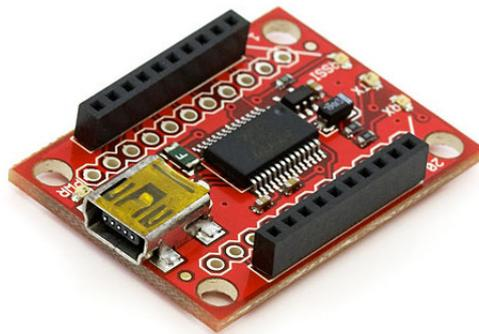
Figura 4.6: XBee Explorer USB.
