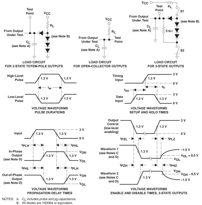
C. Waveform 1 is for an output with internal conditions such that the output is low, except when disabled by the output control.
